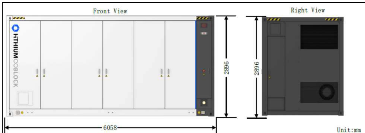
Figure 14: Battery Container Modules: Hithium Block L5015 0.5P V2.0 (Source: ACCIONA Energía)
