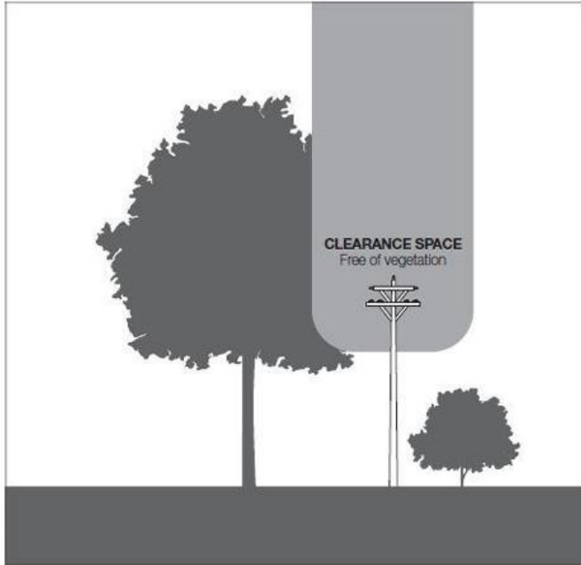
Graph 6—Uninsulated 66 000 volt electric line in a hazardous bushfire risk area
